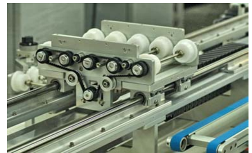
Input Load Module Options Support Cassette or Coin Stack Loading
