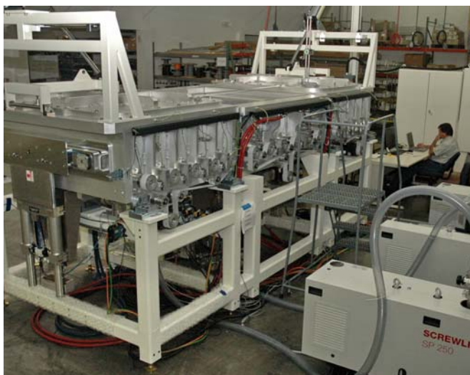
High Vacuum System Undergoing Final Test
