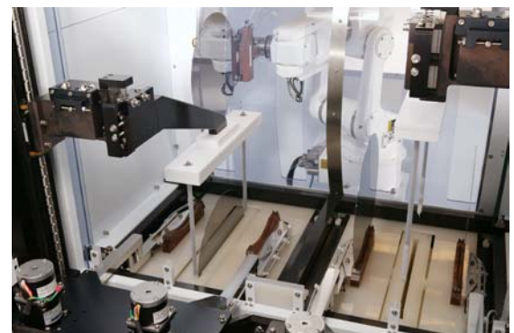
Vertical Edge Grip for Wafer Cleaning Chamber
