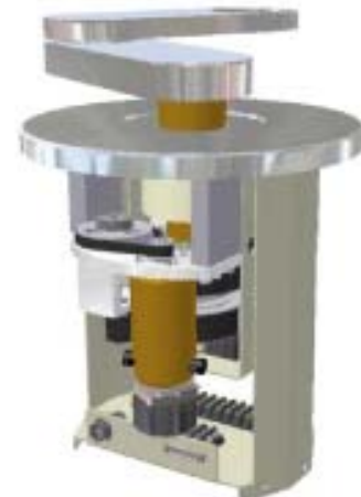
200mm Vacuum Robot Incorporates Ferrofluidic Coupling
