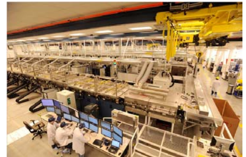
Photovoltaic Processing Line Utilized Many Carrier Transfer Systems Multiplying the Impact Of Tool Reliability Issues
