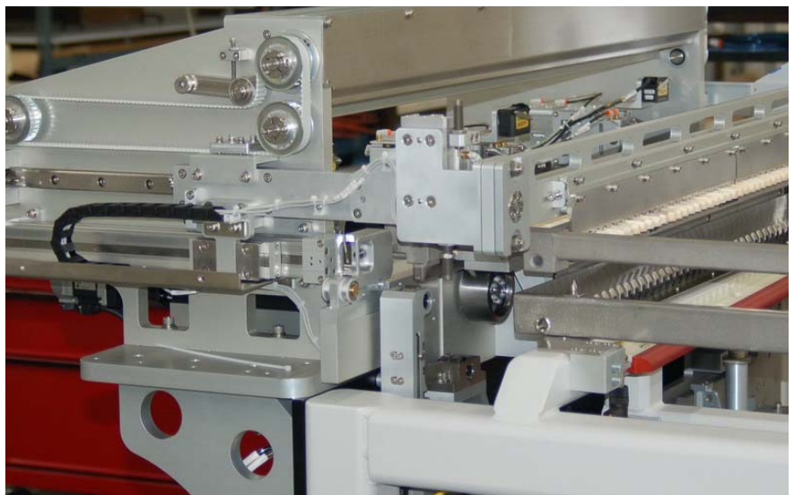
Closeup of Mechanism for Transferring CIGS Glass Substrates
