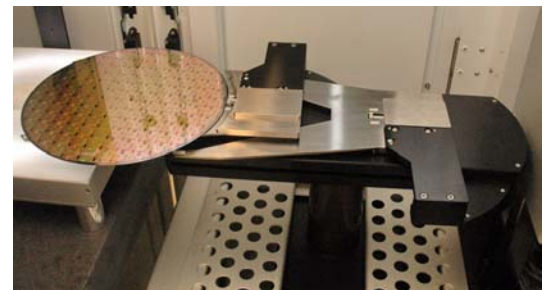
Innovative Wafer Handling Design Accommodates Severely Warped Bonded Wafers
