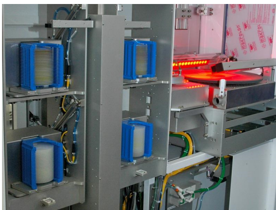
Precision Loading of Wafers into Blind Pockets on Carrier Required
