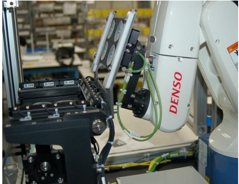
Precision Alignment Tolerances Achieved using Innovative Clamshell Fixturing and Vision Guided Robot
