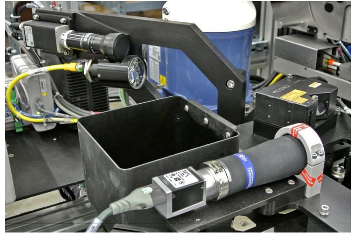
In Process Quality Control Measurement Station Incorporated Off-Axis Illumination
