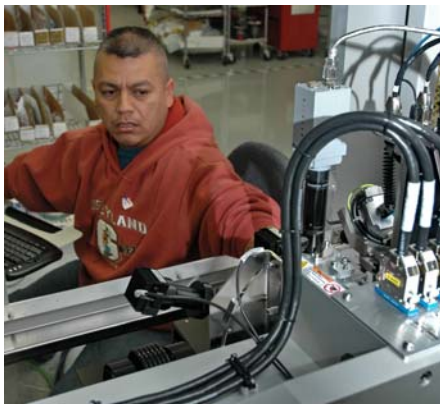
Senior Technician Performing Metrology Head Alignments
