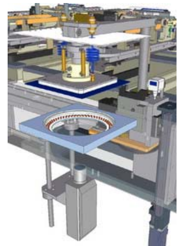
Integrated PV Cell Vision Inspection at Input Station
