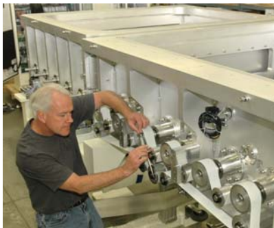
Drive Mechanism Incorporated High Vacuum Feed Throughs
