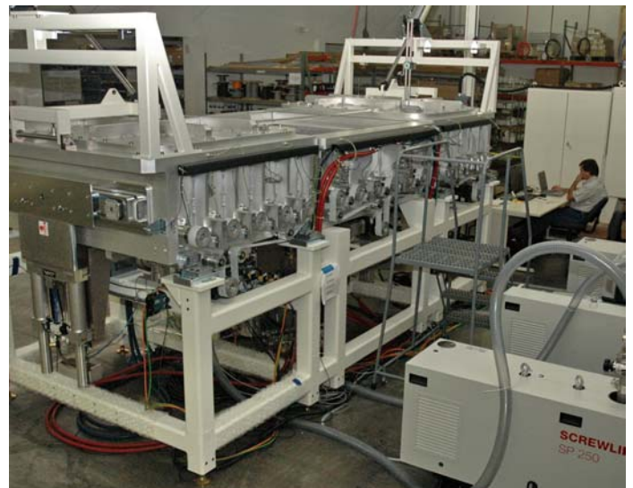
Innovative Drive System Positioned 400 kg Payload Precisely in High Vacuum
