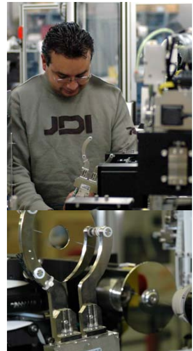
Senior Manufacturing Technician Aligning Edge Grip End Effector
