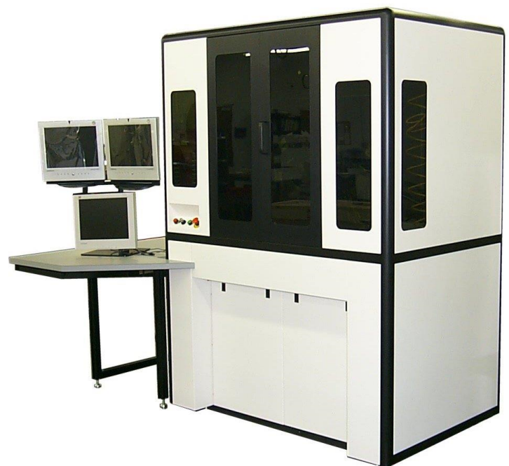
Micropositioning Nd:YAG Fiber Laser Welder for Fiber Optic Transponder
