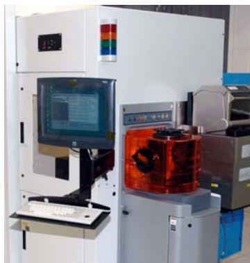
EFEM Supports 200 mm and 300 mm Wafers
