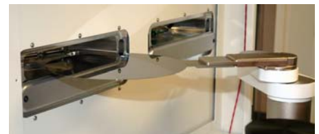
Wafer Hand-off to Vacuum Chamber through Slit Valves
