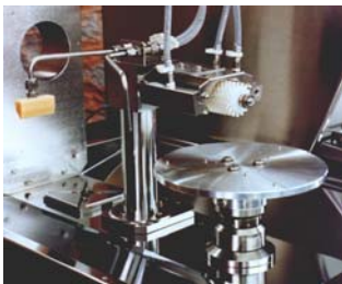
Brush Tower Showing Nitrogen Nozzle
