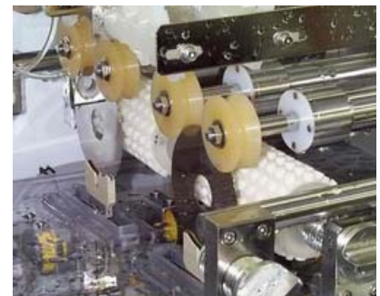
Innovative Media Drive Design (Outer Brush Removed for Clarity)
