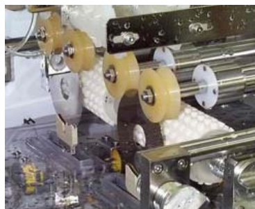
Innovative Media Drive Design (Outer Brush Removed for Clarity)
