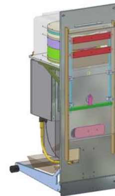
Internal View Showing Load Doors
